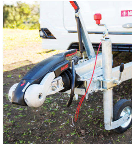
Above: The AL-KO anti-sway hitch and mechanical override brakes mean nearly any car with a tow-ball can tow this caravan easily.
